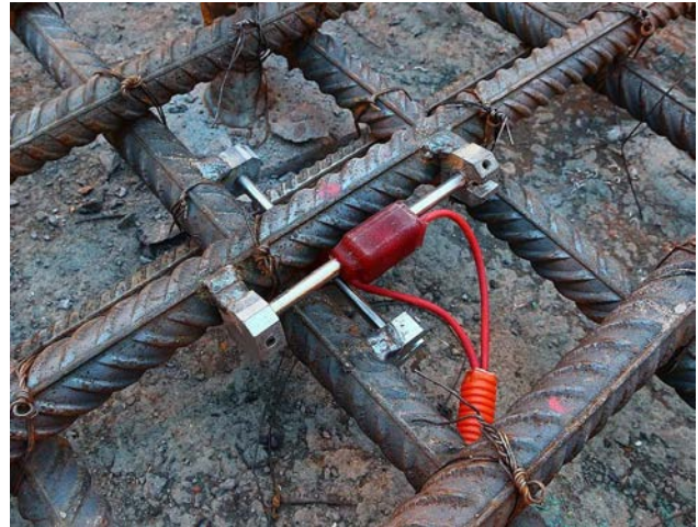
Fig. 9: VW strain gauges installed on the reinforcement of BF bottom plate
