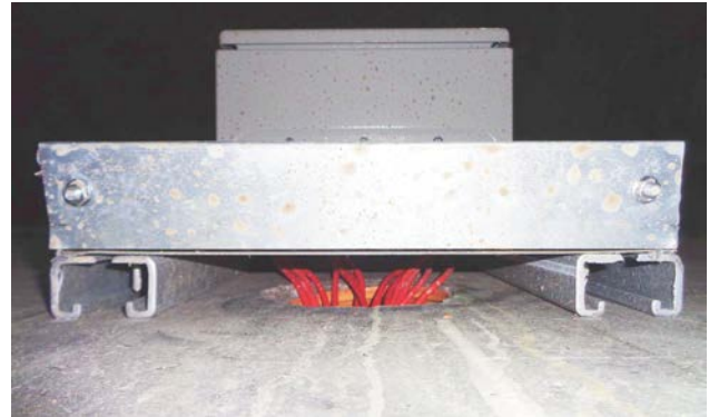
Fig. 16: Multiplexer enclosure installed above the embedded detail with gauge cables
