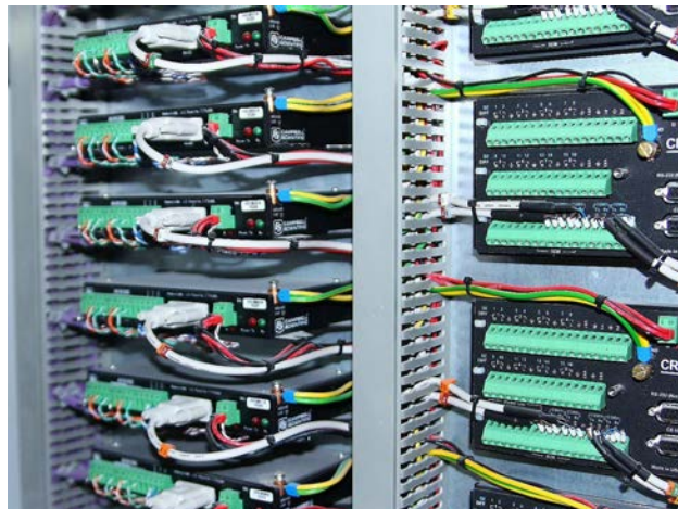
Fig. 15: Typical contents of data acquisition enclosure
